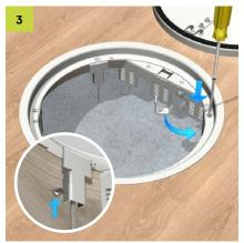
**Claw fastener** Fit the provided claw fastener with the appropriate screws in the frame and tighten them.
