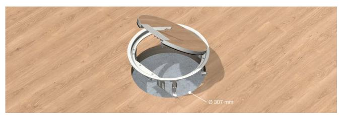
Cartridge installation units with a protective floor covering frame made out of stainless steel, round, with an outside diameter = 330 mm, for hollow space or false floors, with a clamping range from 40 to 80 mm. Usable for floor coverings with a thickness of 12 mm.
