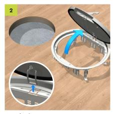
**Opening lever** Open the opening lever behind the cable outlet. Lift the cover outover the rear and the hinge out over.
